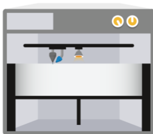
The process continues, building up the part layer by layer
