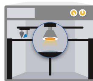
Lamps pass over the surface constantly, the jetted material captures and distributes the heat
